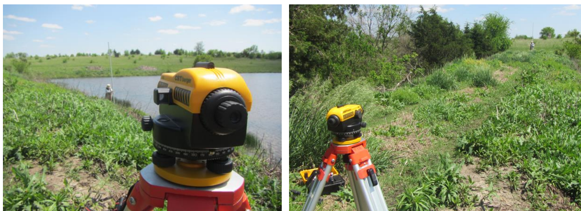
Figure 5. Standing on top of the dam at pond 257 to measure stand pipe height (left) and dam high point (right) relative to water level.
