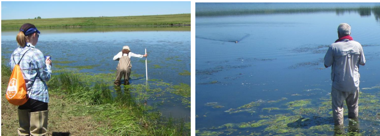
Figure 26. Measuring pond depths around the perimeter with a survey rod (pond 279 left) and remote depth transducer on fishing rod (pond 200 right).
