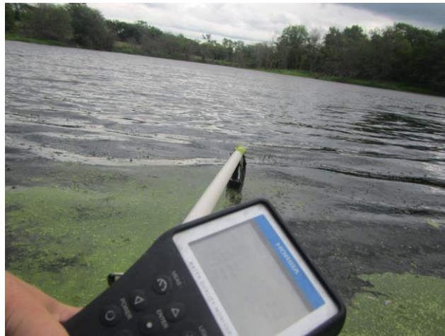
Figure 36. Using a pole to extend the Horiba U-52 water quality monitor beyond the aquatic vegetation at pond 23.
