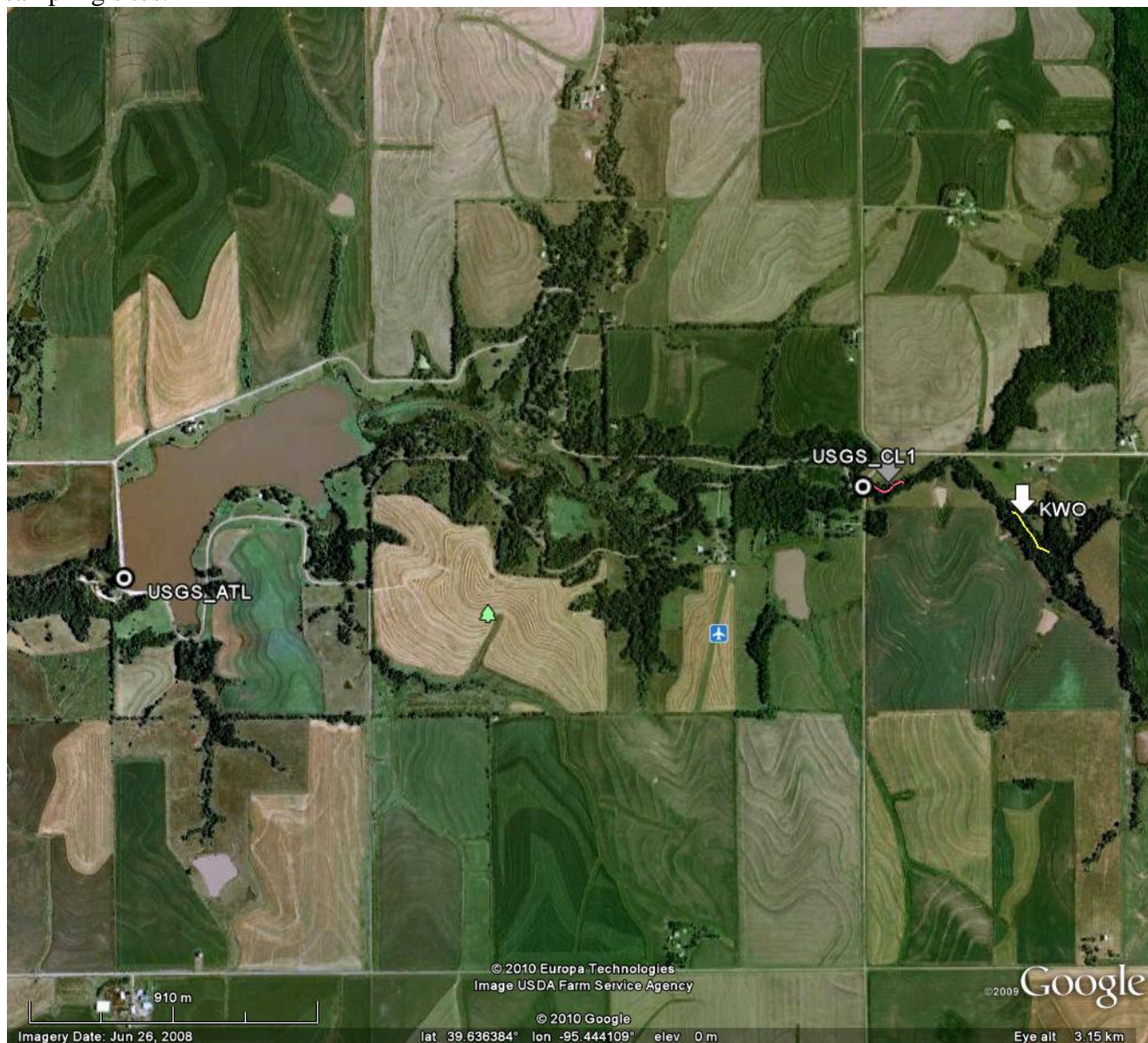
Figure 1. Atchison County Lake showing USGS gaging stations ATL and CL1 and CPCB's (pink) and KWO's (yellow) survey reaches on Clear Creek.
