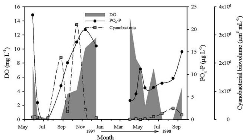
Figure 9. Monthly changes of bottom DO levels and PO<sub>4</sub>-P concentrations in relation to cyanobacterial biovolume at Clinton Lake.
