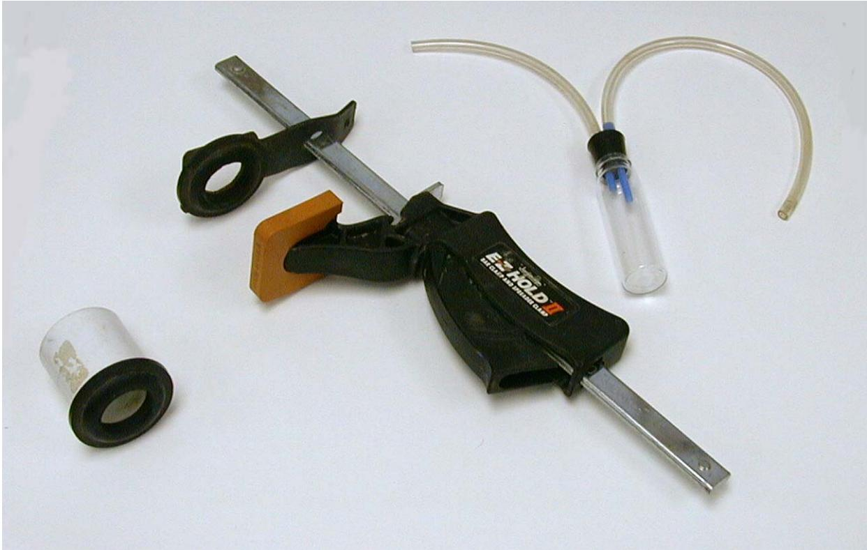
**Figure 1: Original sampling devices used by the CPCB during the 2000 sampling season (from left to right; PVC sampler, bar clamp sampler & aspirator)**
