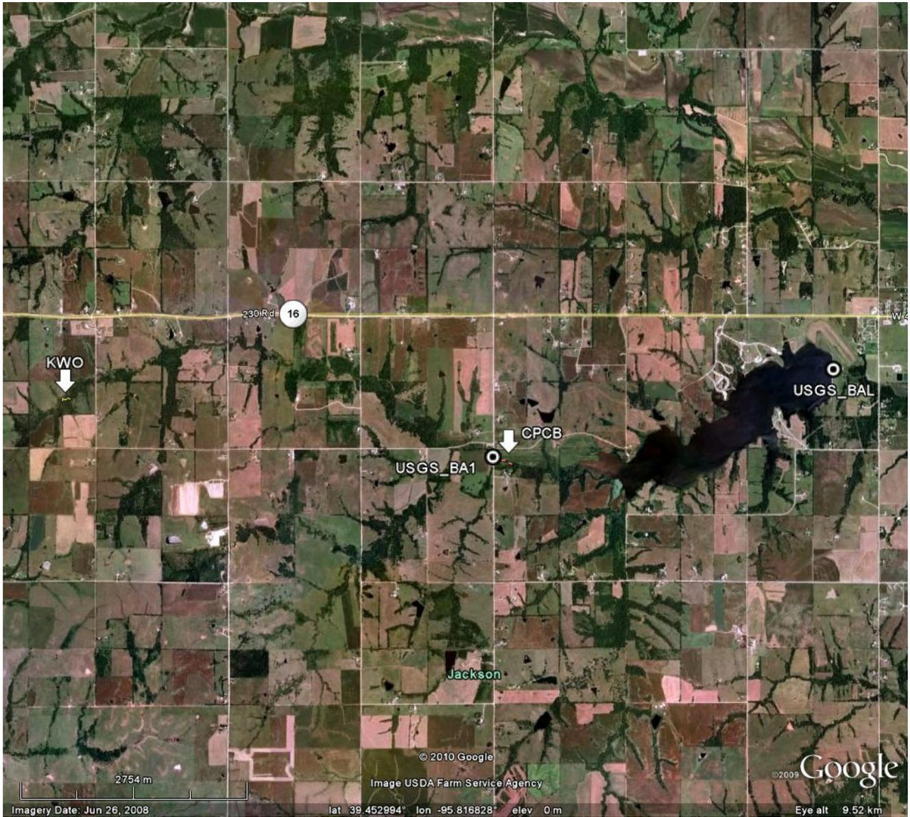
Figure 2. Banner Creek Lake showing showing USGS gaging stations BA1 and BAL and CPCB's (pink) and KWO's (yellow) survey reaches on Banner Creek.
