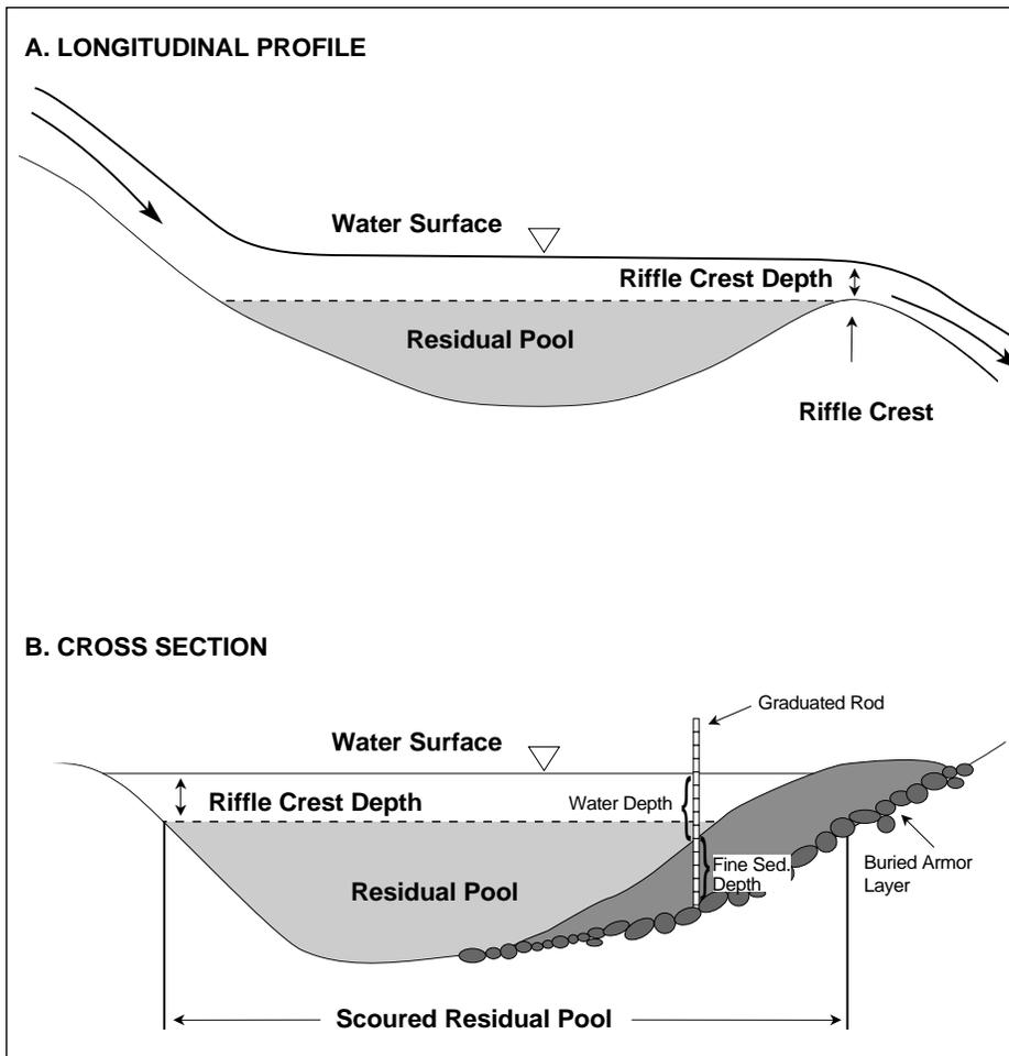
**Figure 1**—(A) Longitudinal profile of a pool, showing the riffle crest and the area included in the residual pool volume. (B) Cross section of a pool, showing measurement of water and fine sediment depth and volume of water and fine sediment in the scoured residual pool.
