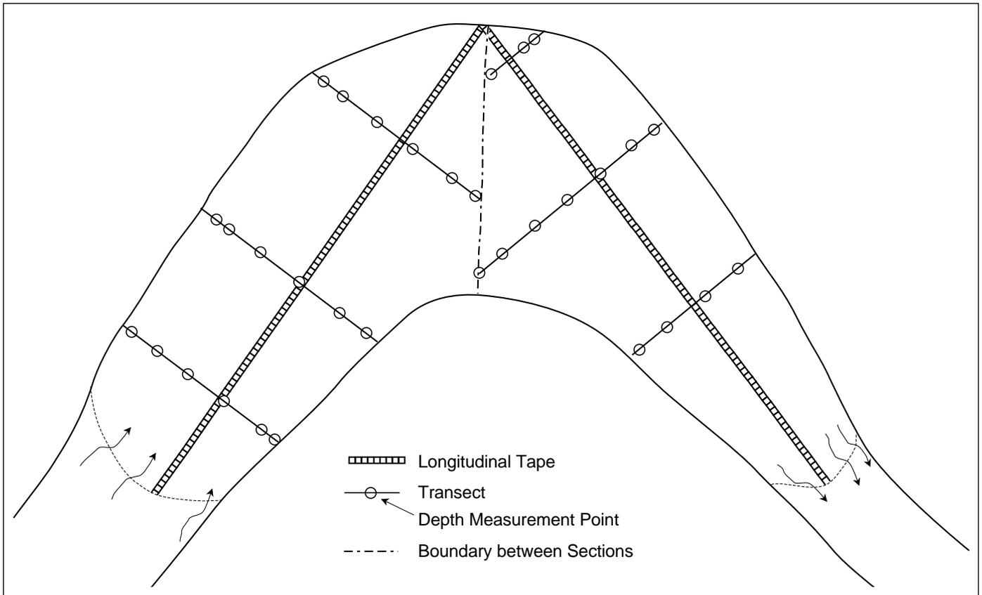
**Figure 3**—Measuring a pool with a bend. The longitudinal tape is strung in two straight segments, transects are located systematically along the tape, and a zero-area cross section is recorded at the location of the bend in the tape.
